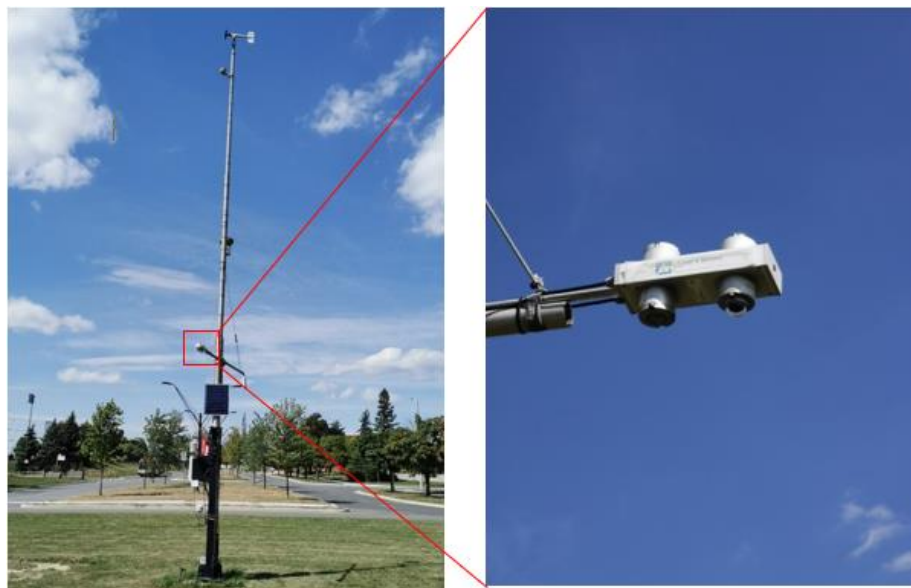
Figure 3: EMOS York University weather station (left) and solar and far infrared radiation balance radiometers (right), (image taken by: Prof. Chen)
